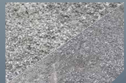
Screened asphalt fractions
