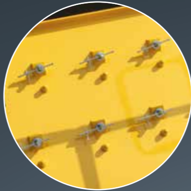
Wedge clamping system Rapid and user-friendly screen change.
