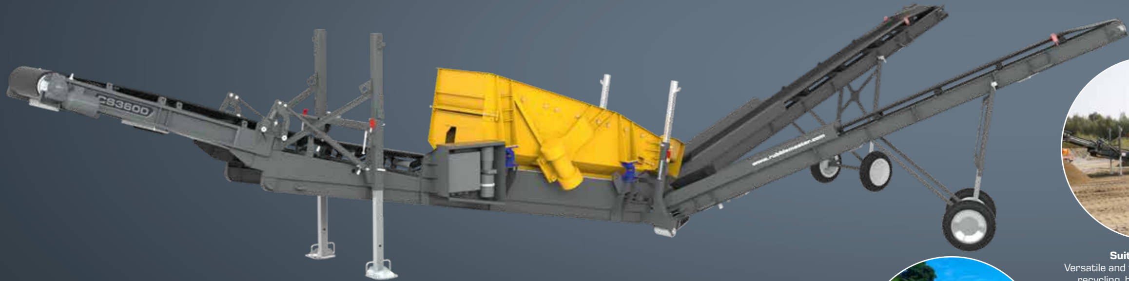
Plugs in to crusher Enormous energy savings due to screener being powered by crusher.
