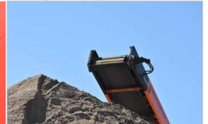
A scraper on the top of the stockpiler, cleans the belt from the material that stick to the belt and simultaneously increases the efficiency of material transfer
