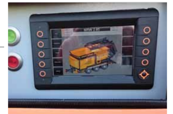
Central control panel with touchscreen
