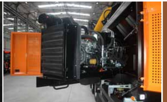
The engine and hydraulic system are mounted on a pull-out frame which provides easy access for maintenance
