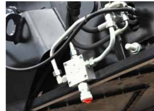
Conveyor belt speed rate adjustment
