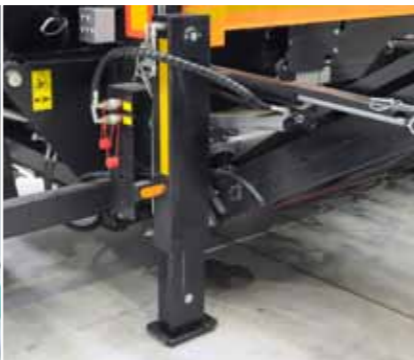
Hydraulic support legs improve machine stability on uneven ground
