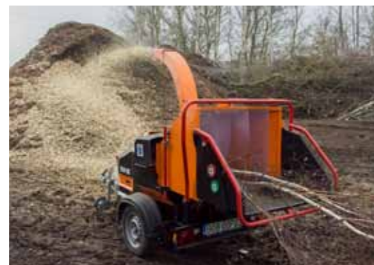
Loading ramp and safety bar.
