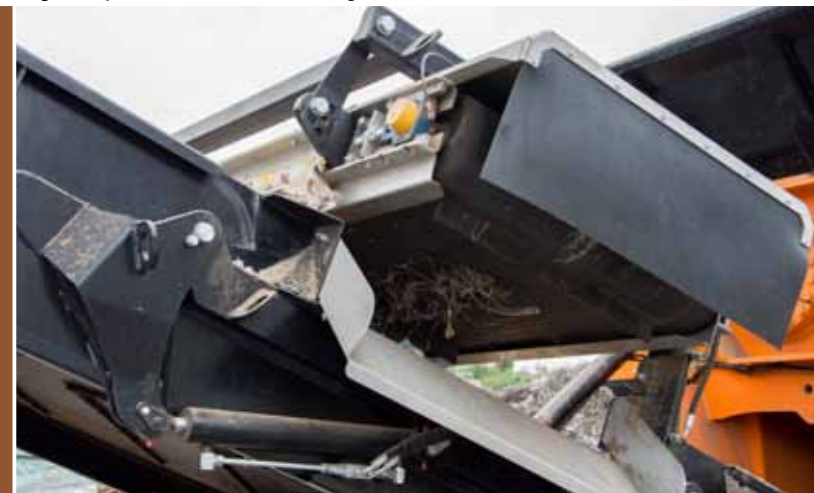
Magnetic separator for extraction of ferromagnetic materials.
