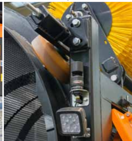
Multifunctional beacon signaling the operating mode Work lamp
