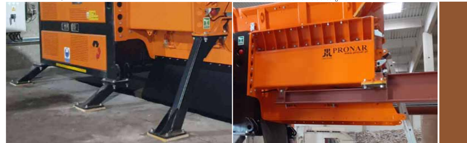
Metal feet for mounting the machine to the floor
