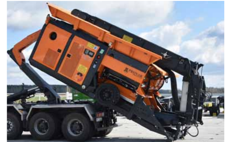
Hooklift standard. Machine designed with easy transport in mind on a three-axle truck thanks to low weight (~16 000 kg).
