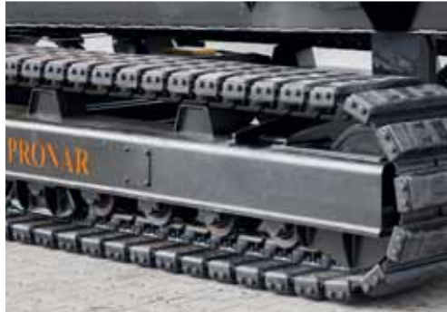
Rubber track pads protect the ground against the scratches
