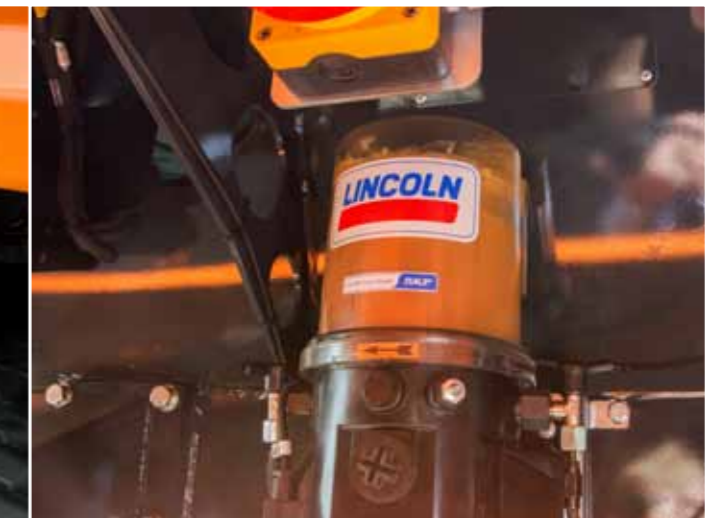
Central lubrication system Provides automatic lubrication of all key machine components.
