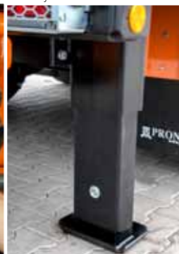
Hydraulic support legs ensures stability of machine
