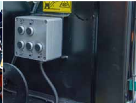
Rear control panel for safe and easy conveyors unfolding.
