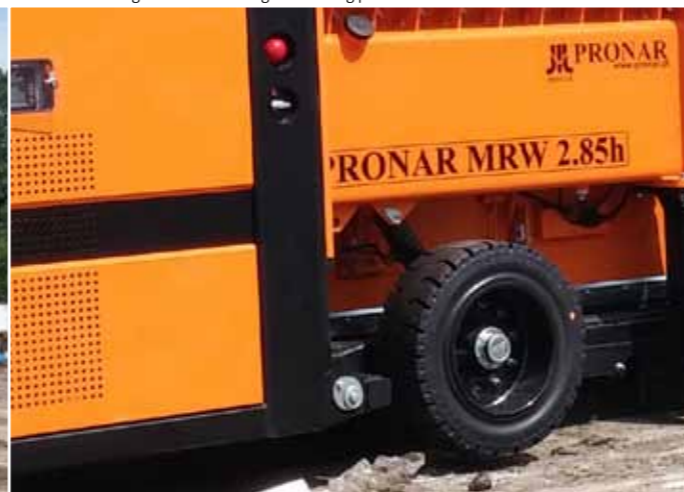
MRW 2.85h - drag wheel for moving on working place
