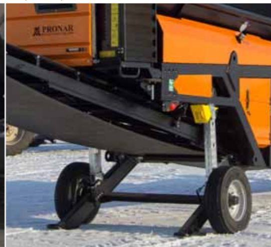
Rear support arm hydraulically adjustable to working or transportation position
