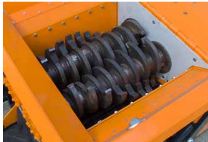
Asynchronous gearbox. Both shafts work at their maximum capacity with every bite.
