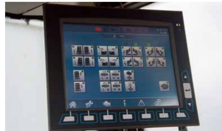
Parking power supply allows to operate the Windrow Turner without starting the diesel engine for service and maintenance
