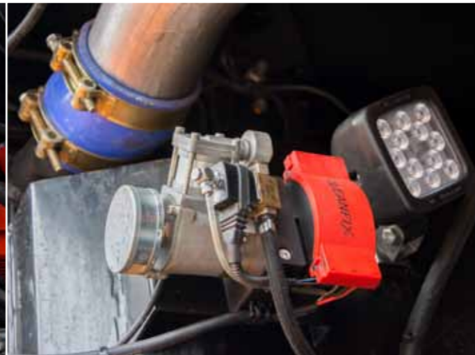
Cleanfix. Facilitates work in difficult conditions - automatic cleaning of oil and engine cooler
