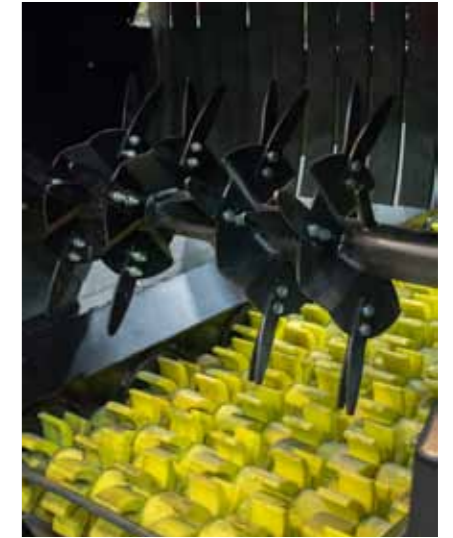
Material spreading shaft
