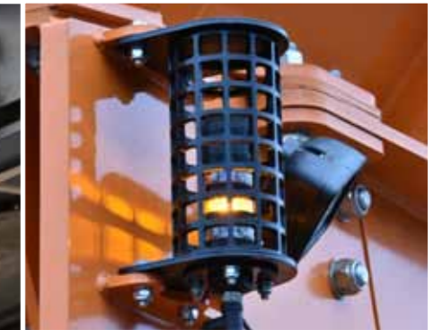
Machine operating mode indicator - for status check and security warnings
